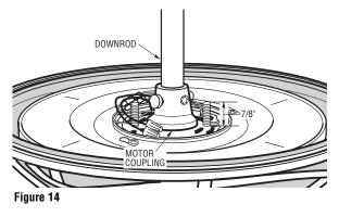
**25.** Slide the motor cover over the downrod and rotate the cover until the threaded studs protrude. Install one lockwasher (supplied) and one knurled knob (supplied) onto each threaded stud to secure the cover to the motor. All wires and wire connectors must be enclosed under the motor cover (Figure15).
